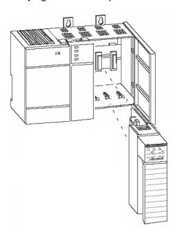
**3** With a firm but steady push, snap the module into place.
